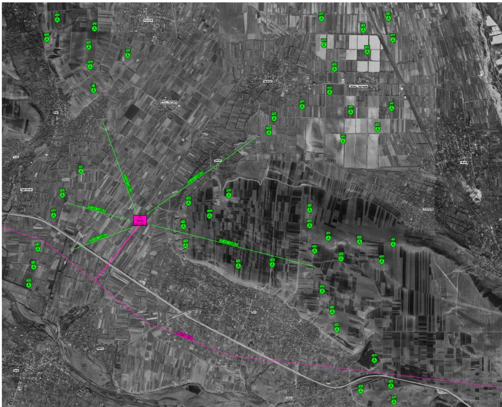
Figure 4-2 Connection to grid: alternative 1
