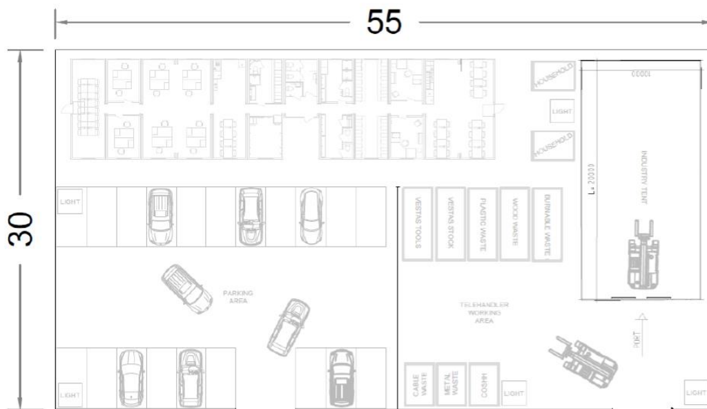
Figure 5-14 Example of site compound for 1 main crane
