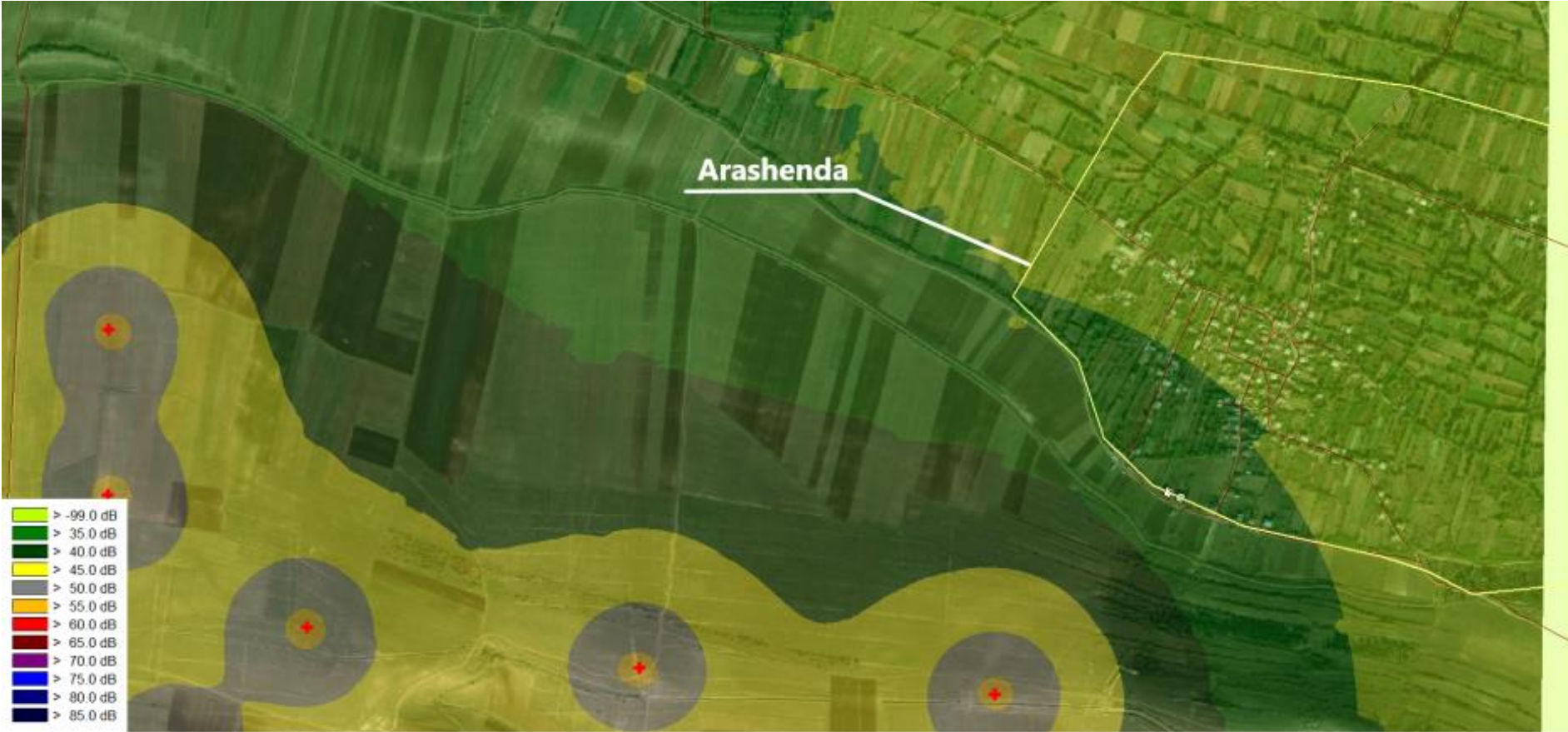
Figure 6-9 Propagation of noise in the vicinity of Arashenda village - Turbine Height - 105 m.
