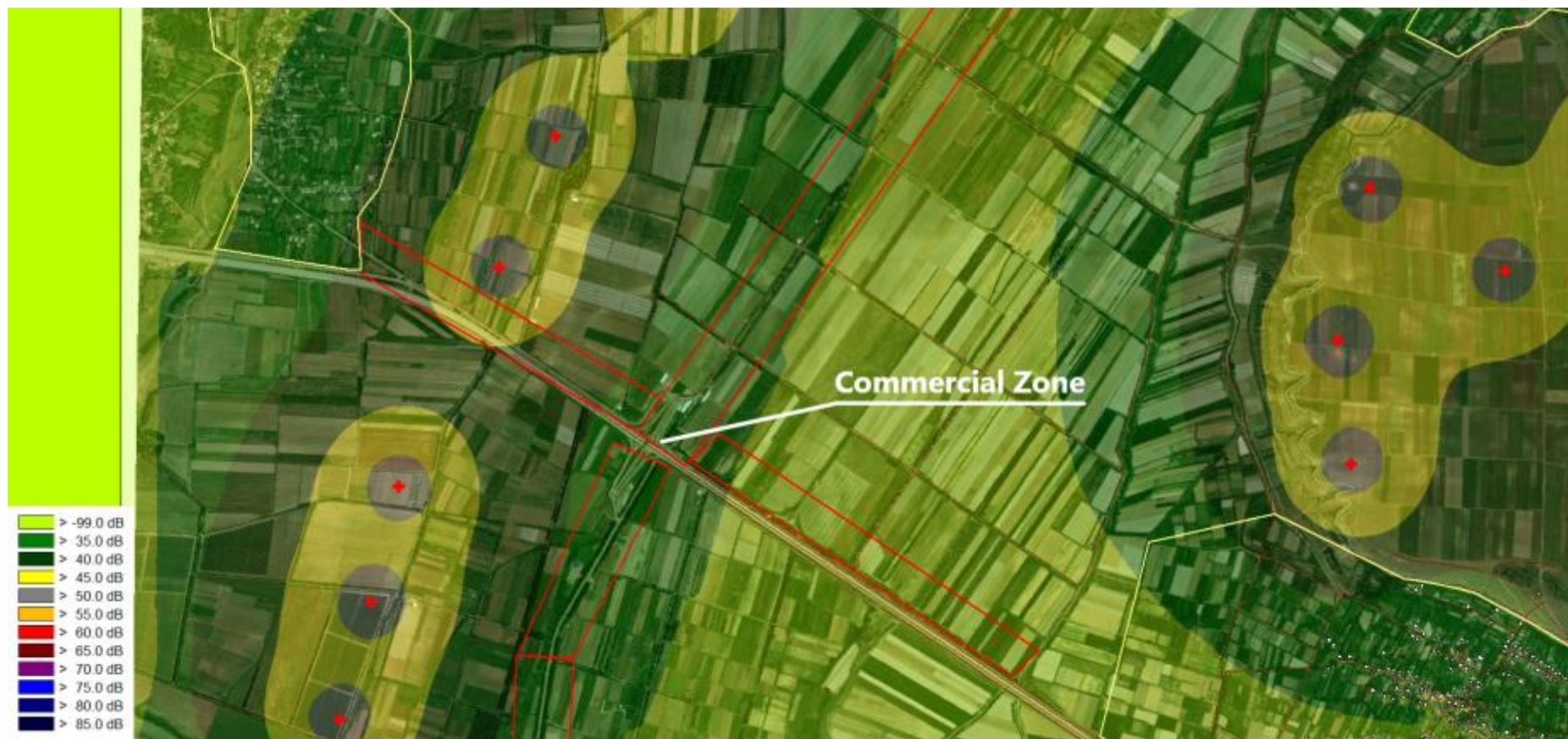
Figure 6-32 Propagation of noise in the vicinity of Commercial zone - Turbine Height - 150 m.
