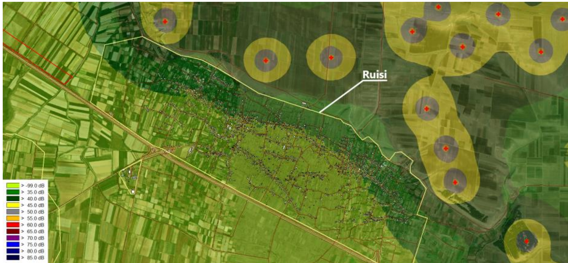
Figure 6-12 Propagation of noise in the vicinity of Ruisi village - Turbine Height - 105 m.
