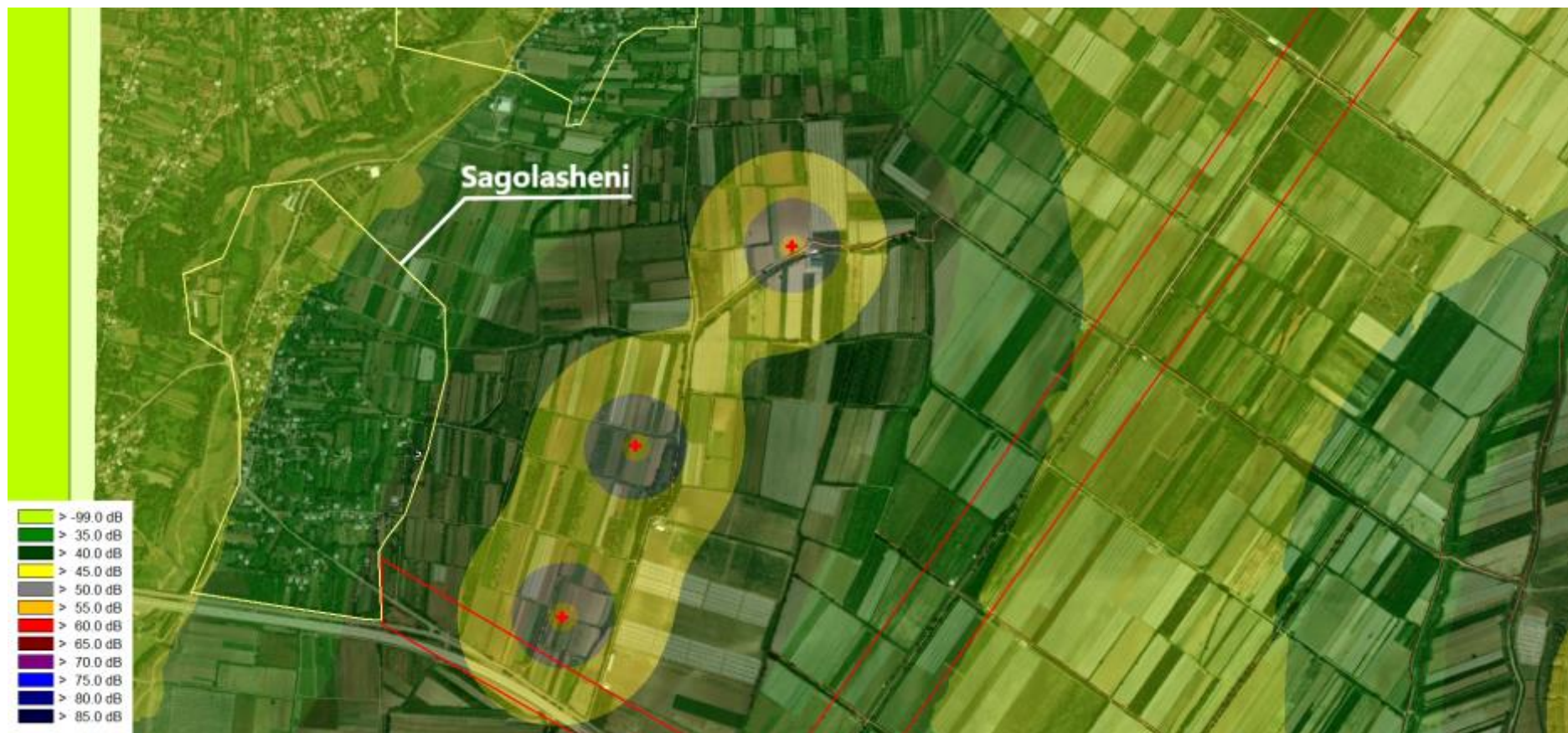
Figure 6-15 Propagation of noise in the vicinity of Sagolasheni village - Turbine Height - 105 m.
