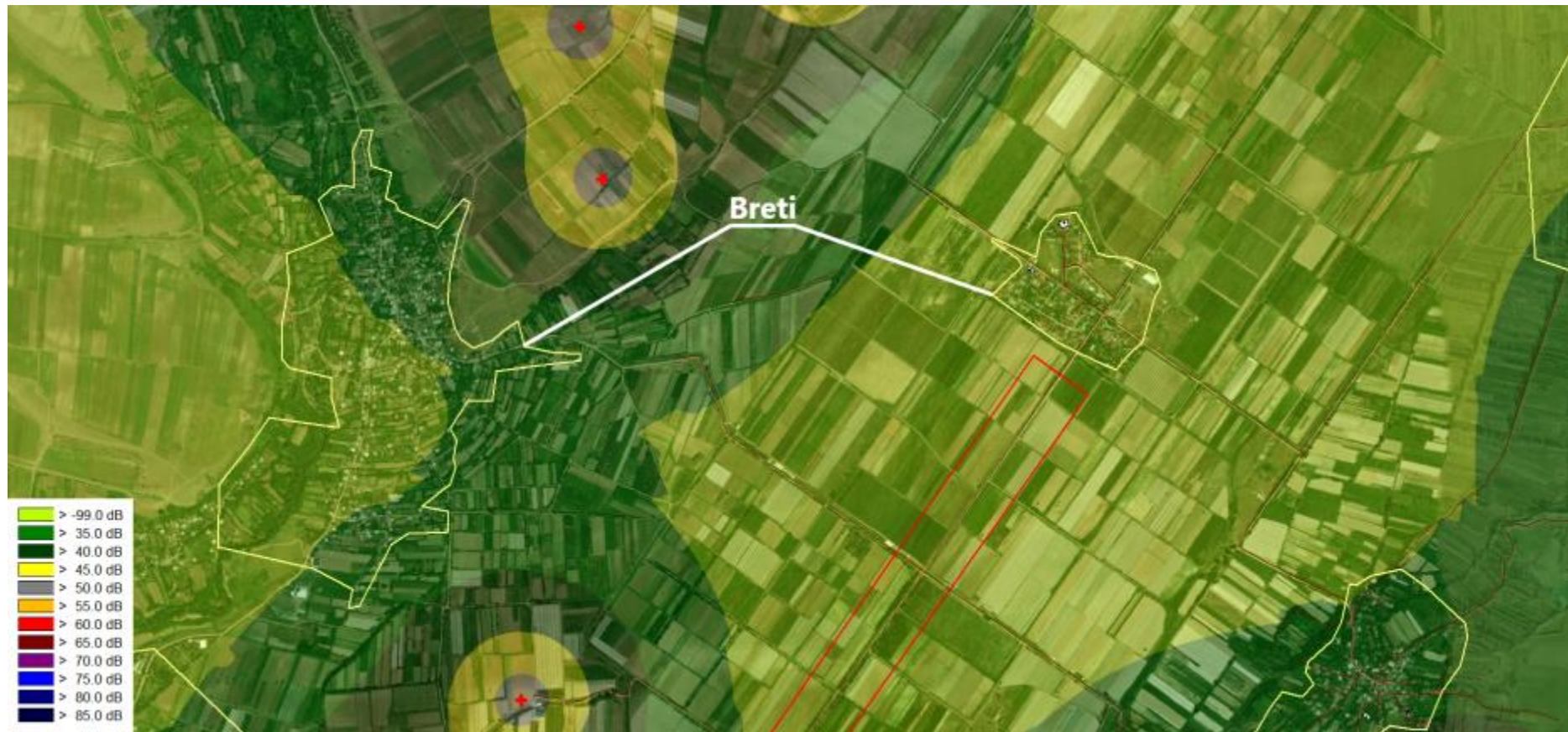
Figure 6-22 Propagation of noise in the vicinity of Breti village and Breti Meurneoba - Turbine Height - 150 m.
