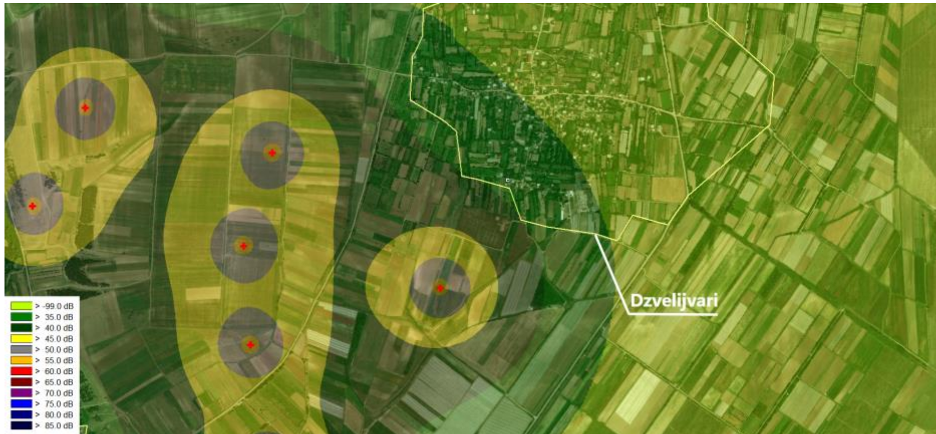
Figure 6-16 Propagation of noise in the vicinity of Dzvelijvari village - Turbine Height - 105 m.
