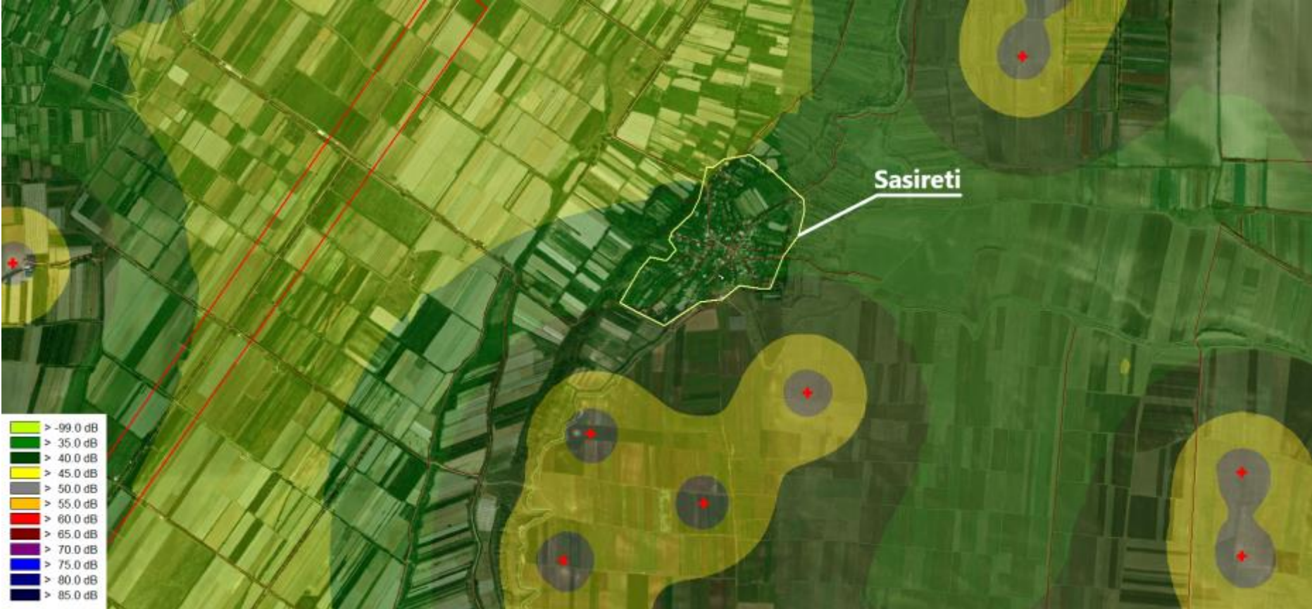
Figure 6-25 Propagation of noise in the vicinity of Sasireti village - Turbine Height - 150 m.
