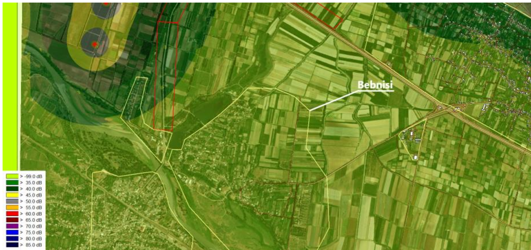
Figure 6-17 Propagation of noise in the vicinity of Bebnisi village - Turbine Height - 105 m.
