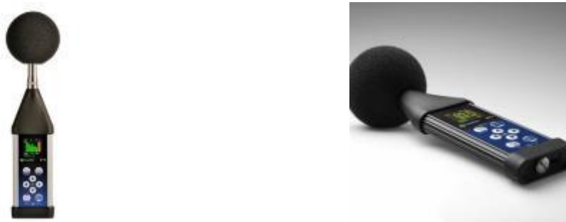
Figure 5-7 Equipment used for noise measuring
