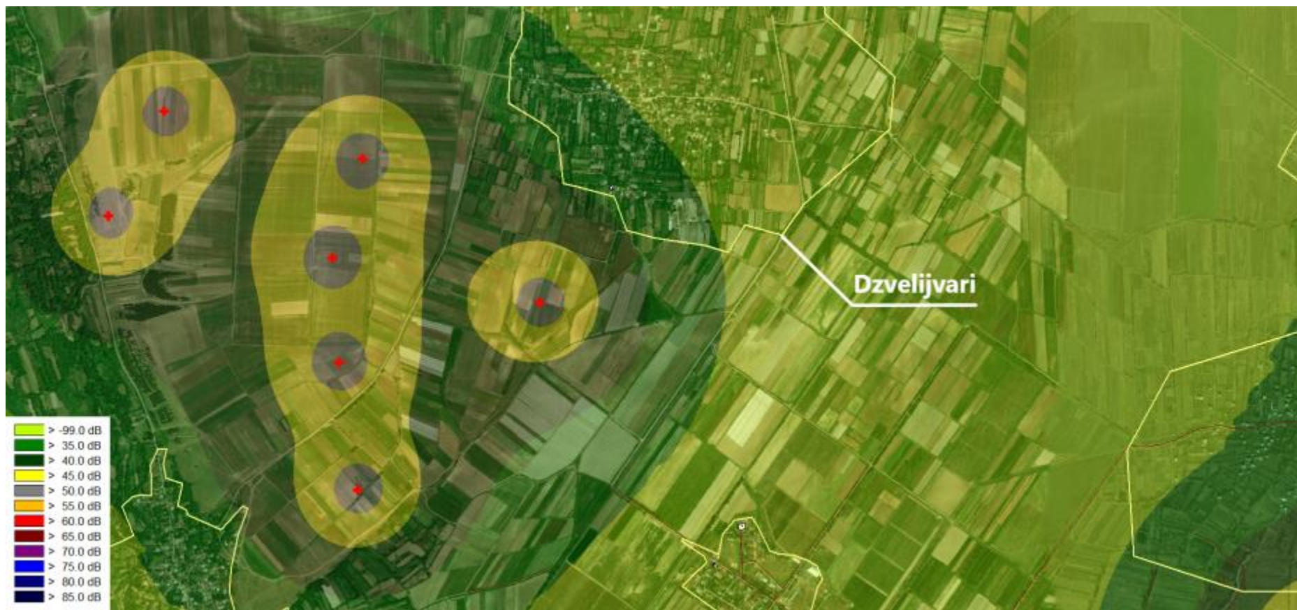
Figure 6-28 Propagation of noise in the vicinity of Dzvelijvari village - Turbine Height - 150 m.
