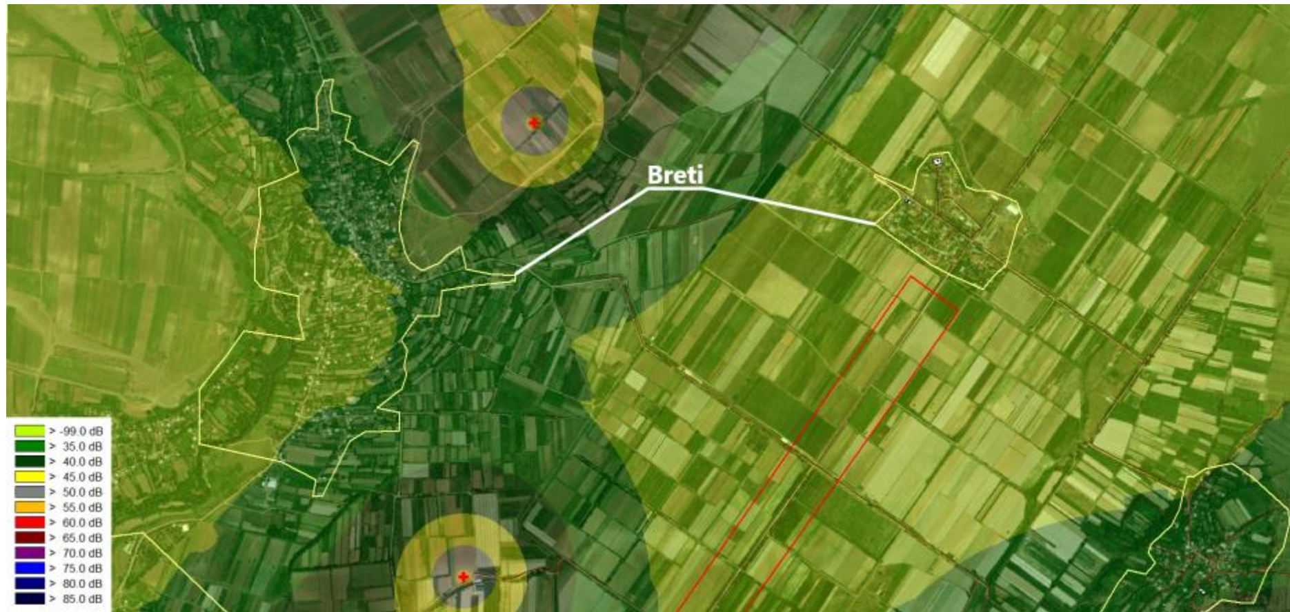
Figure 6-10 Propagation of noise in the vicinity of Breiti village and Breiti Meurneoba - Turbine Height - 105 m.
