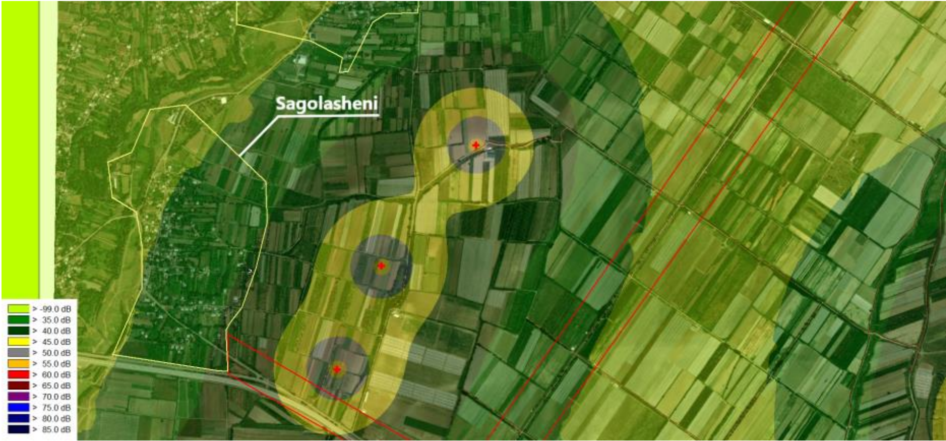
Figure N9.9: Propagation of noise in the vicinity of Sagolasheni village - Turbine Height - 105 m.
