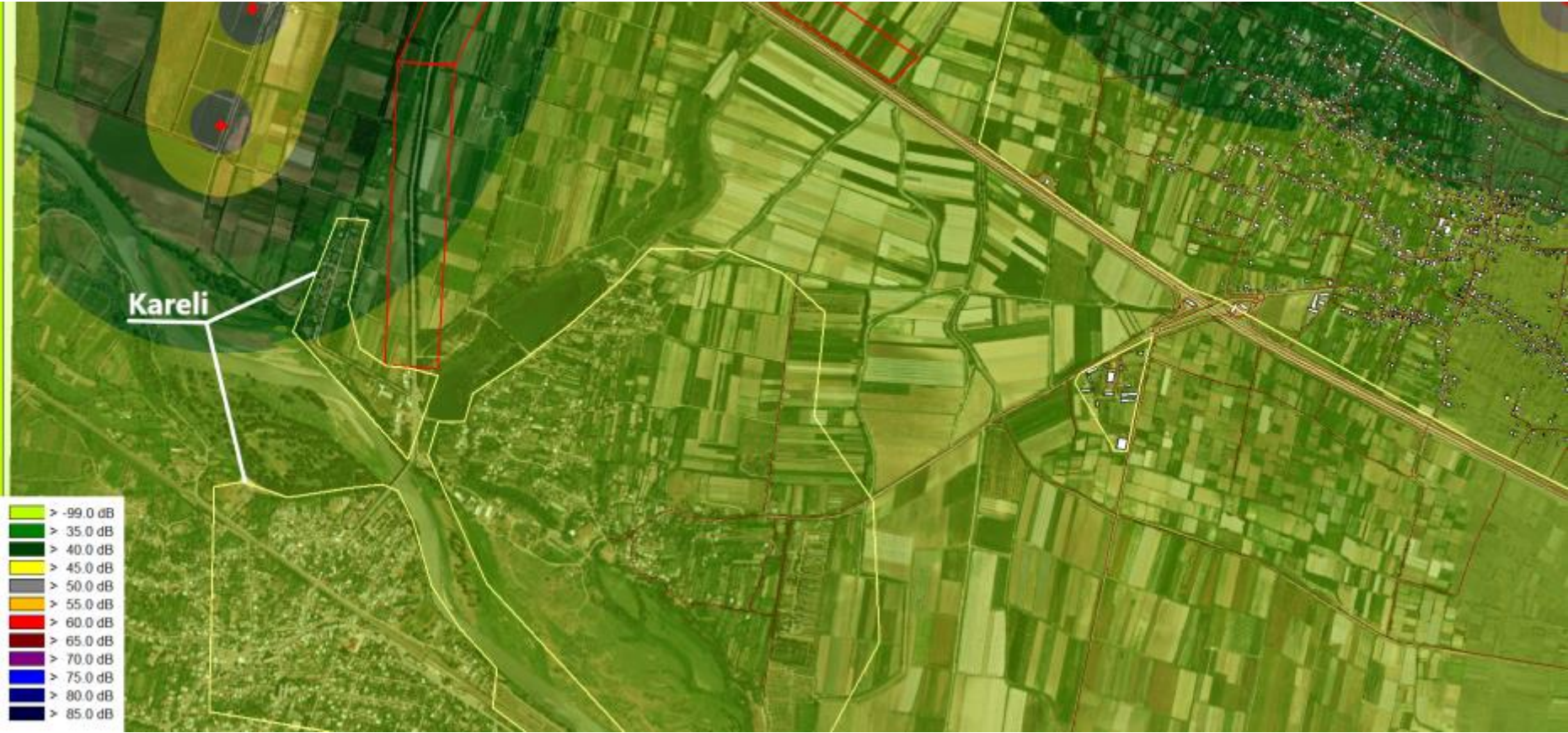
Figure N9.25: Propagation of noise in the vicinity of Kareli - Turbine Height - 150 m.
