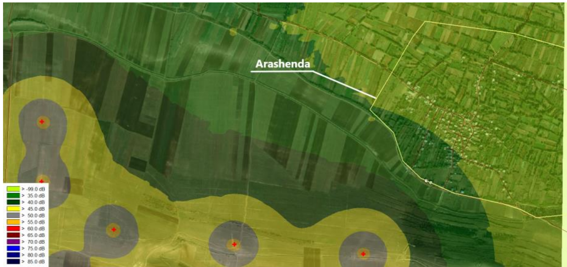
Figure N9.3: Propagation of noise in the vicinity of Arashenda village - Turbine Height - 105 m.
