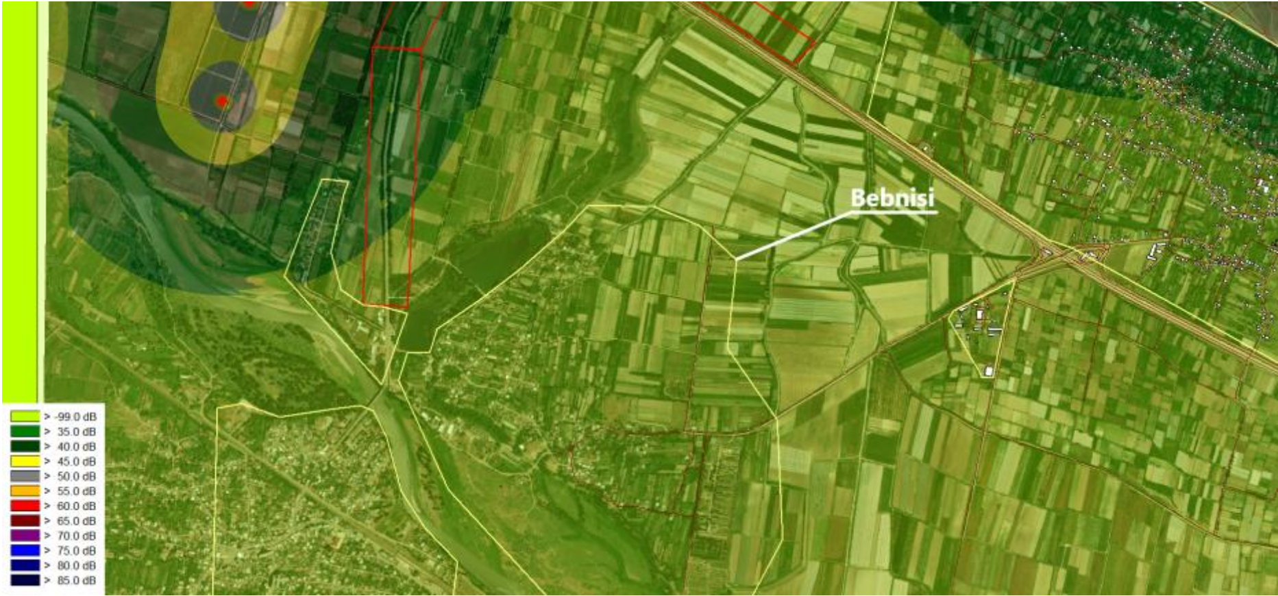
Figure N9.11: Propagation of noise in the vicinity of Bebnisi village - Turbine Height - 105 m.
