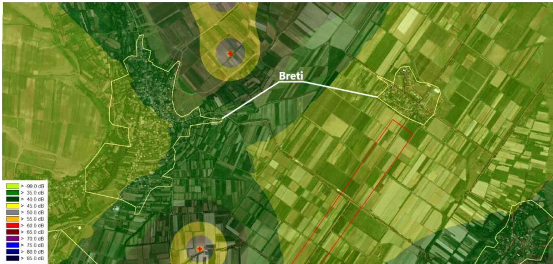
Figure N9.4: Propagation of noise in the vicinity of Breti village and Breti Meurneoba - Turbine Height - 105 m.
