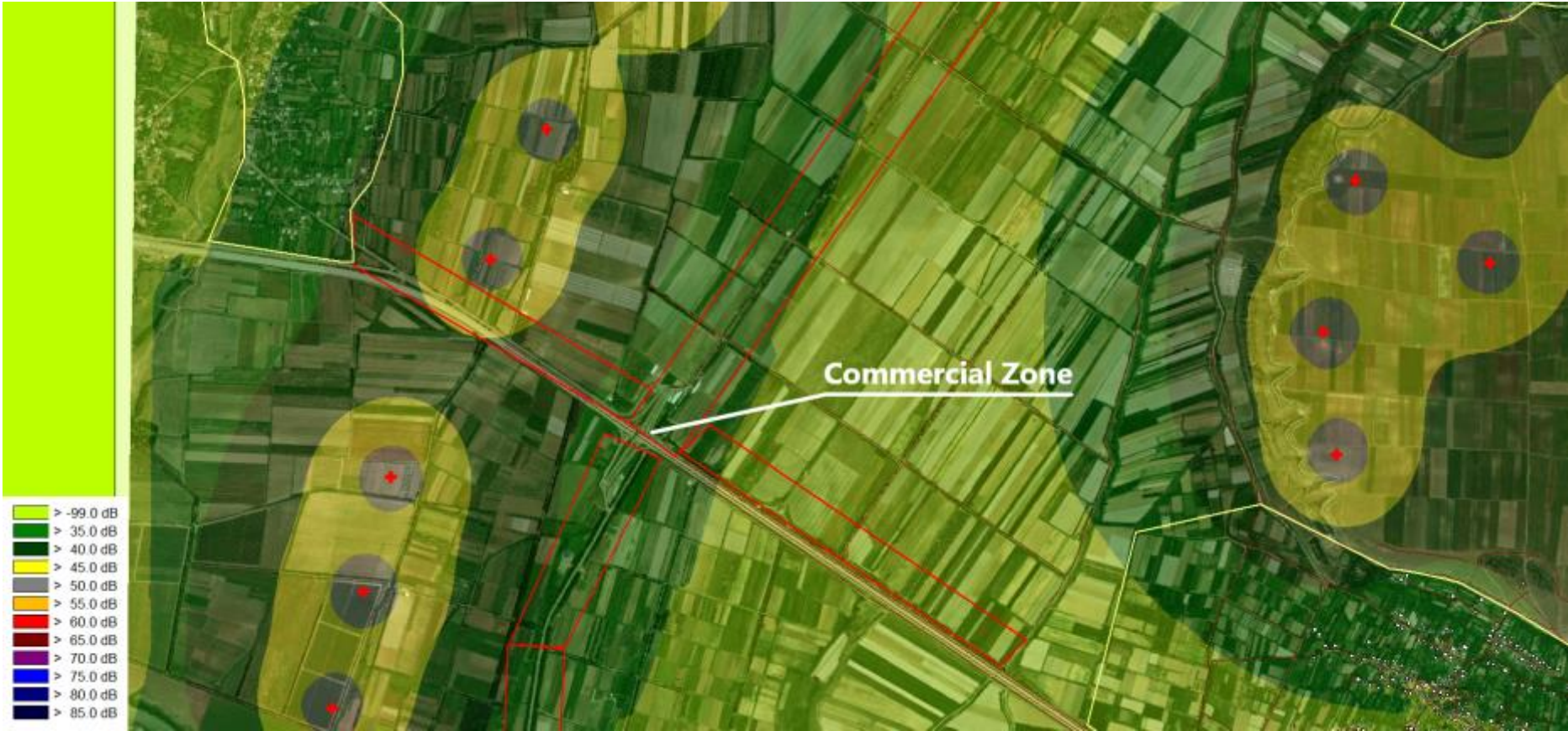
Figure N9.26: Propagation of noise in the vicinity of Commercial zone - Turbine Height - 150 m.
